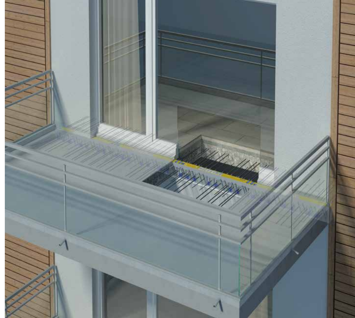
Placement of concrete structural thermal breaks at the balcony window.
