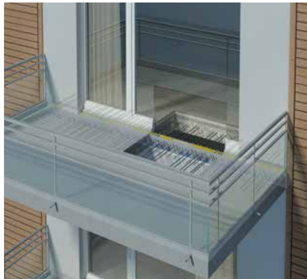
Placement of structural thermal breaks in the balcony to ensure a continuous insulation layer.
