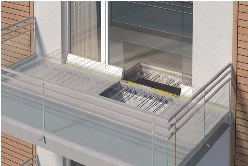
*Placement of Schöck Isokorb® type CM for concrete slab connections in the floor assembly at the building envelope.*
