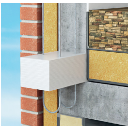
Isokorb® STBs for concrete parapet construction are insulated, engineered assemblies with stainless steel rebar for casting into concrete roof slabs.
