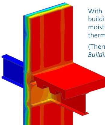
With no thermal break in place, heat and cold can pass through the building envelope at canopy and steel beam connections, causing moisture issues such as condensation and mold and reducing the thermal performance of the building envelope.
