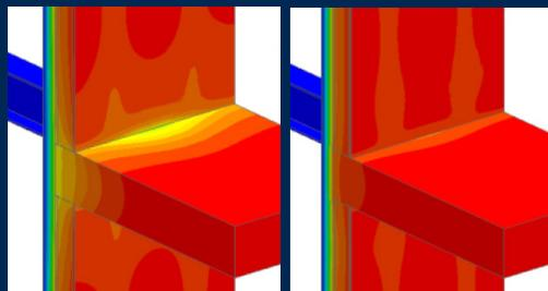
**LEFT:** Standard uninsulated structural connection. Exterior temperature “seeps through” (yellow).
